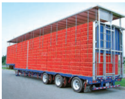
The roof structure on this trailer for transporting live poultry is made of lightweight aluminum for safety, comfort, and durability.
