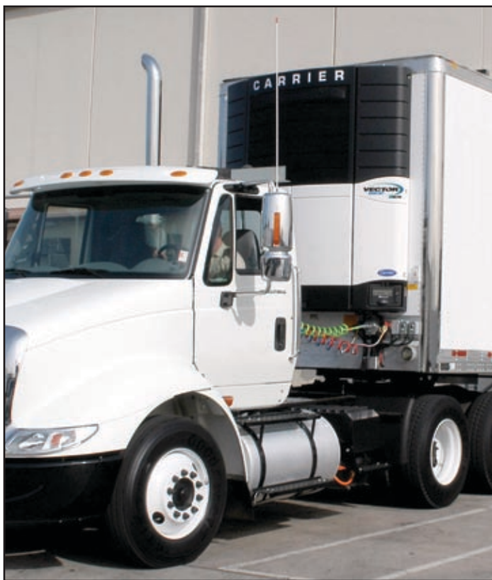
The hybrid Vector 1800MT trailer refrigeration unit offers integrated electric standby capability, providing Canadian operators with a way to significantly cut fuel consumption.
