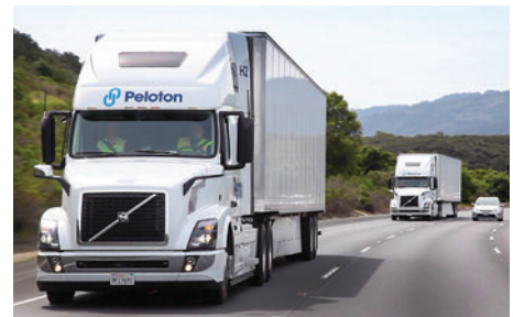
Peloton trucks in a platooning formation – driving with little following distance to reduce drag and increase fuel efficiency. (Photo: Peloton)
